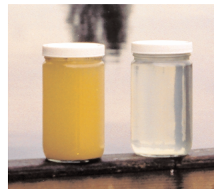
Samples were identical until the right jar was treated with Storm-Klear Gel-Floc.
